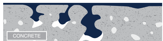
MICROSCOPIC CLOSE UP OF CONCRETE SURFACE USING A SURFACE-COATING SEALER
